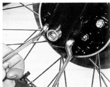
3.4 Settle all components in position and tighten pinch bolt to specified torque setting
