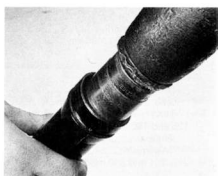
3.8a Tap fork seal into position using a suitable size tubular drift
