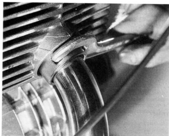
10.3c Tighten ring nut securely – to the specified torque setting if possible
