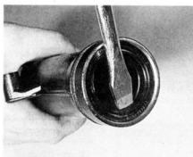
3.6 Take care not to damage lower leg when levering out fork seal
