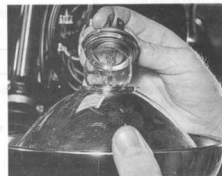
13.2c ...and withdraw the headlamp bulb
