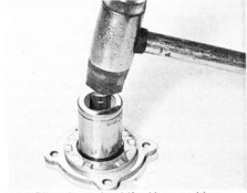
28.4 Oil seals can be drifted into position using a tubular drift
