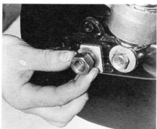
7.2c Remove sprocket cover retaining nut and remove cover from machine
