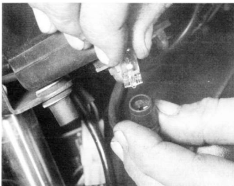
19.2 Instrument illuminating bulbs are a push fit in their holders
