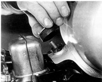
2.6 Do not omit mounting rubbers when refitting fuel tank
