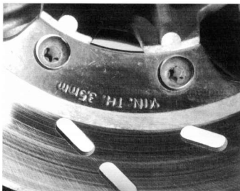
12.4 Service limit is stamped in brake disc flange
