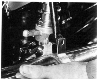
10.3b ... and refit the rear mounting clamp
