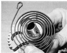
32.1a On 125 and 150 models ensure spring internal tang is correctly located in slot in kickstart shaft
