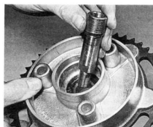
7.7b Refit sprocket spindle to the sprocket ...
