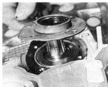
12.3b ... and remove cap ...
