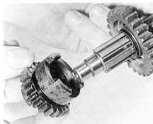
26.8c Slide on the 4th gear pinion ...
