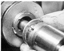
35.1d ... ensuring slot in cam locates with tab on the rotor
