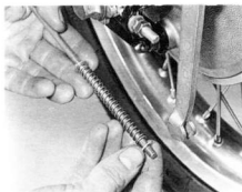
5.2b ... and refit the washers and spring to brake rod
