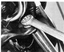
5.3a First tighten both fork top bolts to specified torque setting ...
