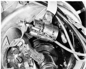
4.1 Condenser (capacitor) is mounted on the stator housing
