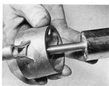
13.2c ... and preload adjuster
