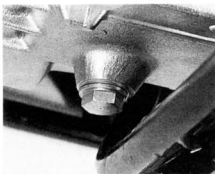
On 250, 251 and 300 models drain plugs are situated on underside of the crankcase ...
