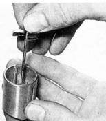
5.3e On all other carburettors needle and retaining plate can be tipped out of valve once cable is disconnected
