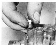
6.4c On 30 N 3-1 carburettor pilot jet is concealed behind threaded plug ...
