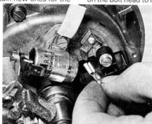
7.2a Disconnect brushholder wires ...
