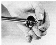
3.9c ... then fit stepped washer, spring and sealing washer to end of damper rod
