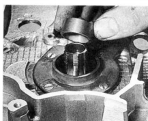
4.7 On 125 and 150 models withdraw spacer from mainshaft oil seal
