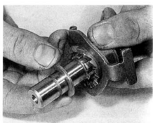
32.3b Fit the camplate to the ratchet and slide on a plain thrust washer ...
