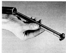
3.9a Lubricate piston ring and insert damper rod into stanchion upper end
