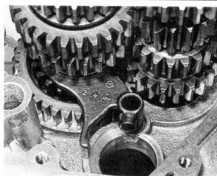
29.6b ... and using notes made on dismantling fit bottom selector fork to the output shaft 4th gear pinion
