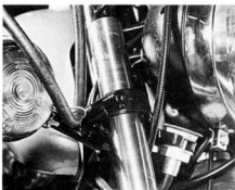
5.1 Refit stanchions to the yokes and refill with specified amount of oil
