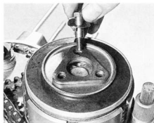
33.7b ... refit the clutch bolts and tab washers, tightening them to the specified torque setting ...
