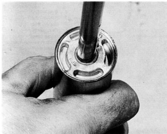
13.4 Threaded ring can be unscrewed using a suitable peg spanner
