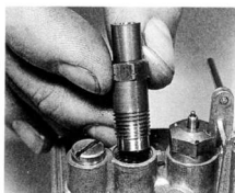
6.4b ... which is a screw fit into carburettor body
