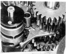
29.6d Fit the centre and top selector forks ...
