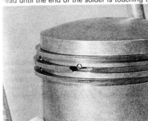
36.1 Ensure piston ring end gaps align with piston locating pegs
