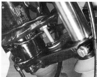
18.3 Headlamp mounting frame attaches to lower yoke by two throughbolts and nuts
