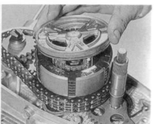
33.5e Refit the pressure plate ...
