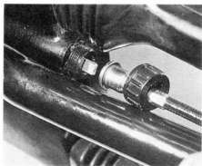
7.2b ... and disconnect speedometer drive cable
