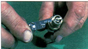
Electrode gap check – use a wire type gauge for best results
