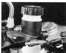
Ensure fluid level is kept between marks on the front of master cylinder reservoir
