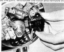
7.2b ... and remove it from stator housing
