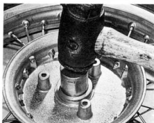
6.6b Drift first bearing into position using a suitable size socket ...
