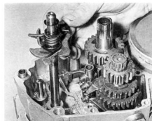
29.5a Refit the gearchange shaft ...
