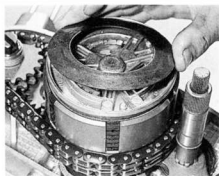
33.5g Fit clutch spring with its convex side facing outwards ...
