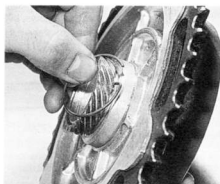
7.7a Ensure speedometer drive gear circlip fits into hole in sprocket
