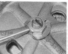
33.9c ... and secure it with the tab washer
