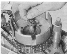
33.3a Fit the thrust washer ...
