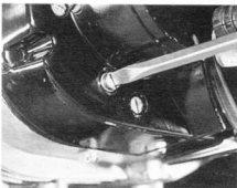
Transmission oil level screw location - 125 and 150 models
