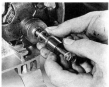
35.1c Fit the cam and rotor retaining bolt ...
