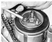
33.7c ... and bend up the tab washers
