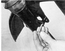
5.4 Refit the mudguard mounting bolts but do not tighten them until front wheel has been fitted
