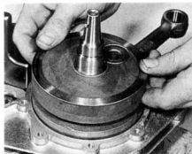
29.1 Do not use excessive force when fitting crankshaft
