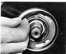
4.8b On 250, 251 and 300 models remove O-ring and clutch adjusting plate
