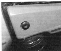
11.9 Tail fairing front mounting
