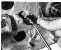
4.8b ... and neutral switch (where fitted)
