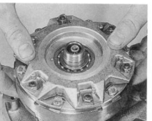
33.12a Refit the clutch assembly
