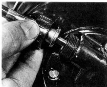
4.8a Unscrew knurled retaining ring and disconnect tachometer cable – 251 shown
