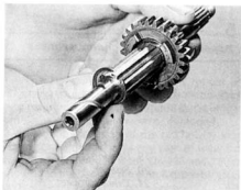
26.6a Take the bare mainshaft slide on the 4th gear pinion and secure it in position with a circlip
