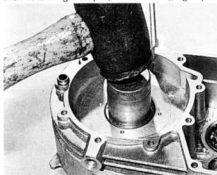
28.2 Tap bearings into place using a suitable tubular drift
