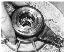
33.13b ... and refit the internal worm gear
