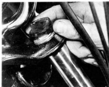
5.3c Refit the plastic covers (where fitted) to fork top bolts ...
