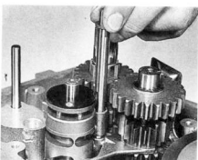
29.6e ... and refit the selector fork shaft
