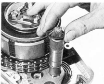
34.1b On 125 and 150 models do not forget to refit thrust washer on kickstart shaft
