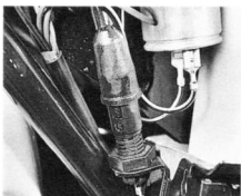
On 251 models rear stoplamp switch is adjusted using plastic sleeve unit ...
