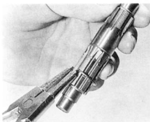
26.7 Fit a circlip to the central groove on the shaft
