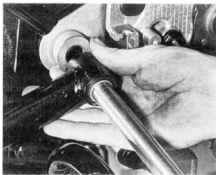
12.2 Do not omit thrust washers when refitting swinging arm
