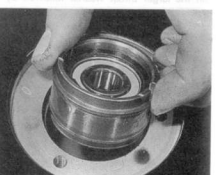
33.13a Fit the external worm gear to the casing ...
