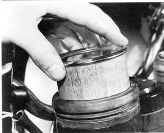
16.1a To remove instrument head, disengage it from its rubber cover ...
