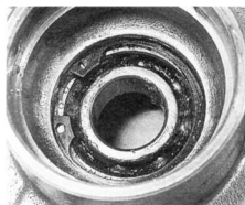
7.4 On 125 and 150 models, sprocket is fitted with single bearing, retained by circlip
