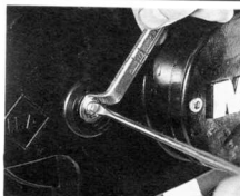
Adjusting clutch lifting mechanism – 125 and 150 models
