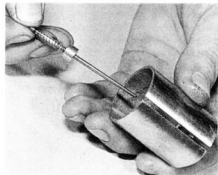
5.3d Needle assembly can then be withdrawn from top of throttle valve
