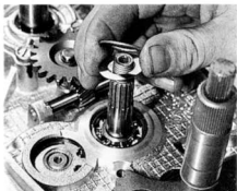
33.1a Refit the thrust washer, shims (where fitted) ...
